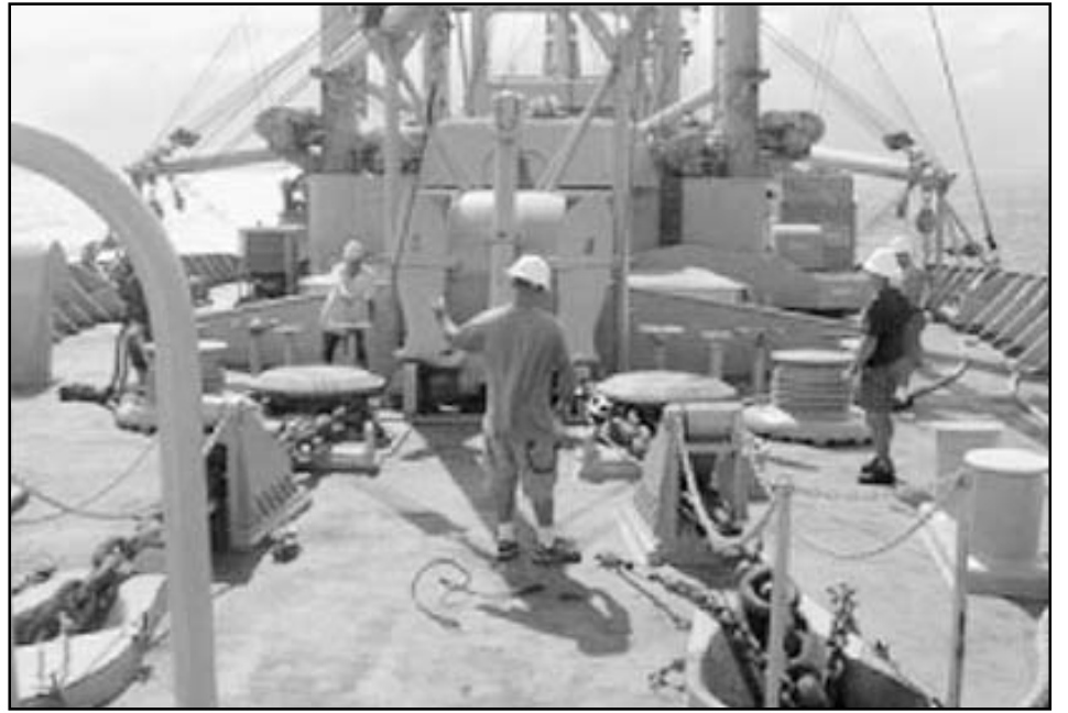
Bosun Brian Yost in the Cape Jacob on August 10, bringing the port anchor home with the ship's cargo gear. The Jacob is a Ready Reserve Force vessel operated by Matson Navigation Company for the Military Sealift Command.
