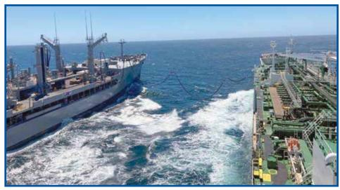
July 11-14 2020 – Off the coast of Southern California Military Sealift Command's long-term chartered motor tanker ship Empire State (T-AOT 5193) conducted connected at-sea refueling operations (CONSOL) with three MSC **Combat Logistics Fleet ships.**
