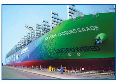
TEU container ships, including the Jacques Saadé class which were the first large LNG-fueled containership ships. CSSC's shipyards built a total of nine of the vessels which each have a capacity of just over 23,000 TEU.
