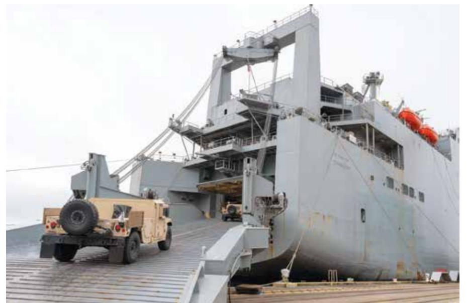
Heavy equipment ramp capable of handling 2 1-A1 Abrams tanks at once.
