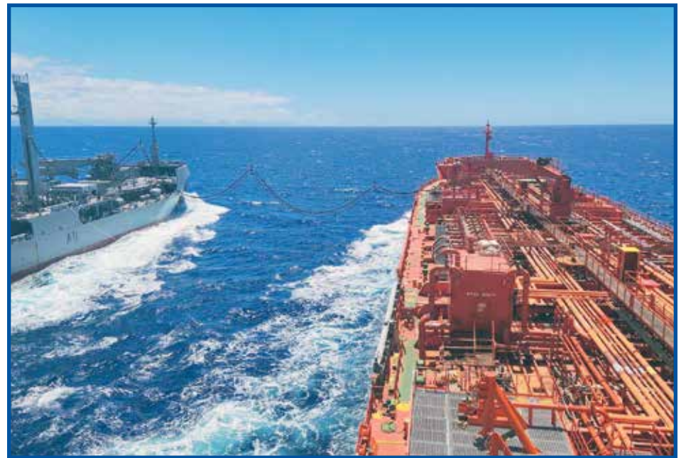
The conventional tanker Allied Pacific rigged with CONSOL gear engaged in strategically important underway replenishment during the RIMPAC exercise off Hawaii last month. The ship is crewed on deck by members of the Sailors' Union of the Pacific.
