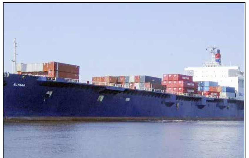
El Faro was built in 1975 at Sun Shipbuilding & Drydock Company in Chester, Pennsylvania, as the Puerto Rico . She was renamed Northern Lights in 1991 and finally El Faro in 2006. On her fateful last voyage, the 790-foot vessel was carrying 391 containers and 294 trailers and cars, plus 33 mariners.
