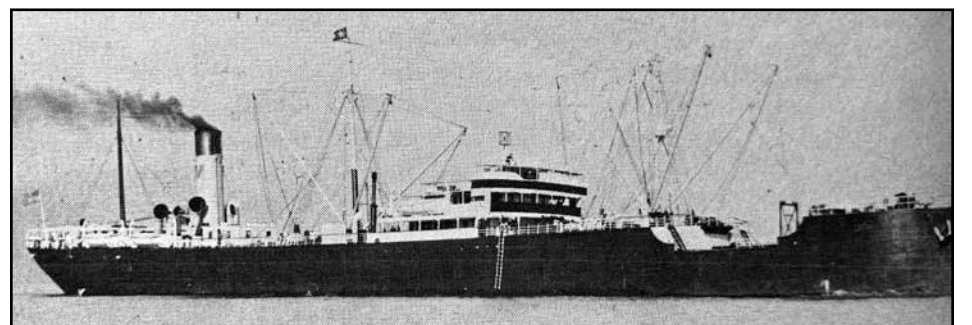
To free the midship section for cargo, the Matson Navigation Co. built a number of steamers with their engines aft until the 1920's. Here is the first steamer Lurlne , a 5,928 ton sugar and general cargo carrier built in 1908. She had limited passenger accommodations under the bridge amidships. (Courtesy Morton-Waters Co.)
