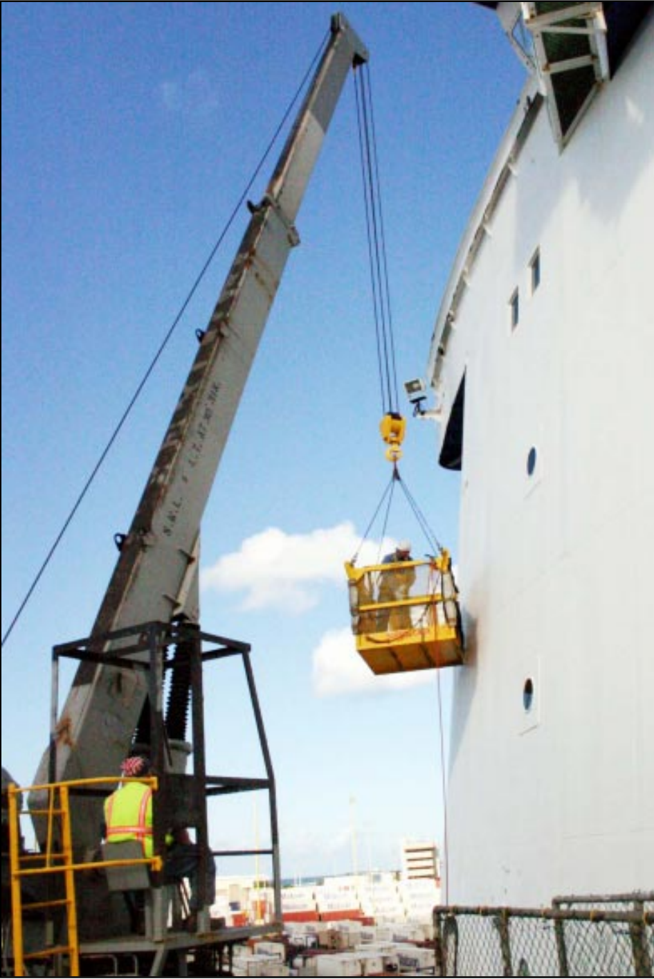
AB Dmitri Seleznev in the basket painting the face of the house in Matson Navigation Company's Mahimahi at sea on May 20. AB and delegate Mick McHenry is operating the crane. Photo: Chris Bujnowski.
