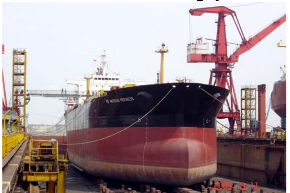
The SeaRiver American Progress sits on the blocks in the drydock at Keppel Shipyard in Singapore.
